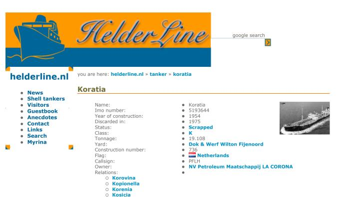
• 1975 scrapped Pusan. Turbo Electric Propulsion System.
